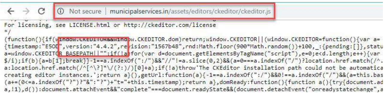
Figure I3: The application uses CKEDITOR version 4.4.2 which has publicly known vulnerabilities.
